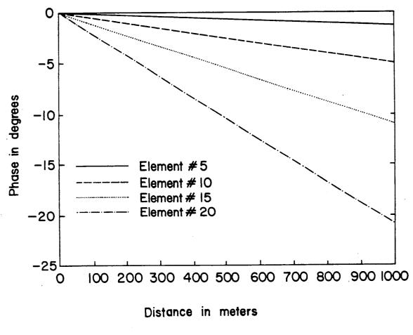
Phase Corrections to move focal point from 60Km to 61Km
