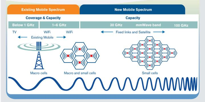
Mobile spectrum showing the radio frequency range from 3-100 GHz with new 5G spectrum above 6GHz. Other radio services (TV, Wi-Fi, Fixed links & Satellite) are shown for reference.
