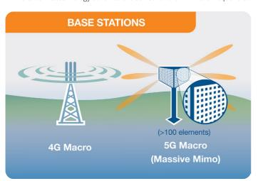
4G sector base station and 5G base station with a new multi element Massive MIMO antenna array. The overall physical size of the 5G base station antenna is expected to be similar to a 4G base station antenna.
