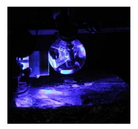
Blue light (465 nm) is used to convert  $CO_2$  to alcohols with a substituted pyradine catalyst and a p-GaP electrode.
