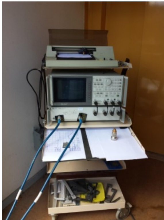
Figure 3. Hewlett and Packard Network Analyzer model 8753C used for return loss and isolation measurements
