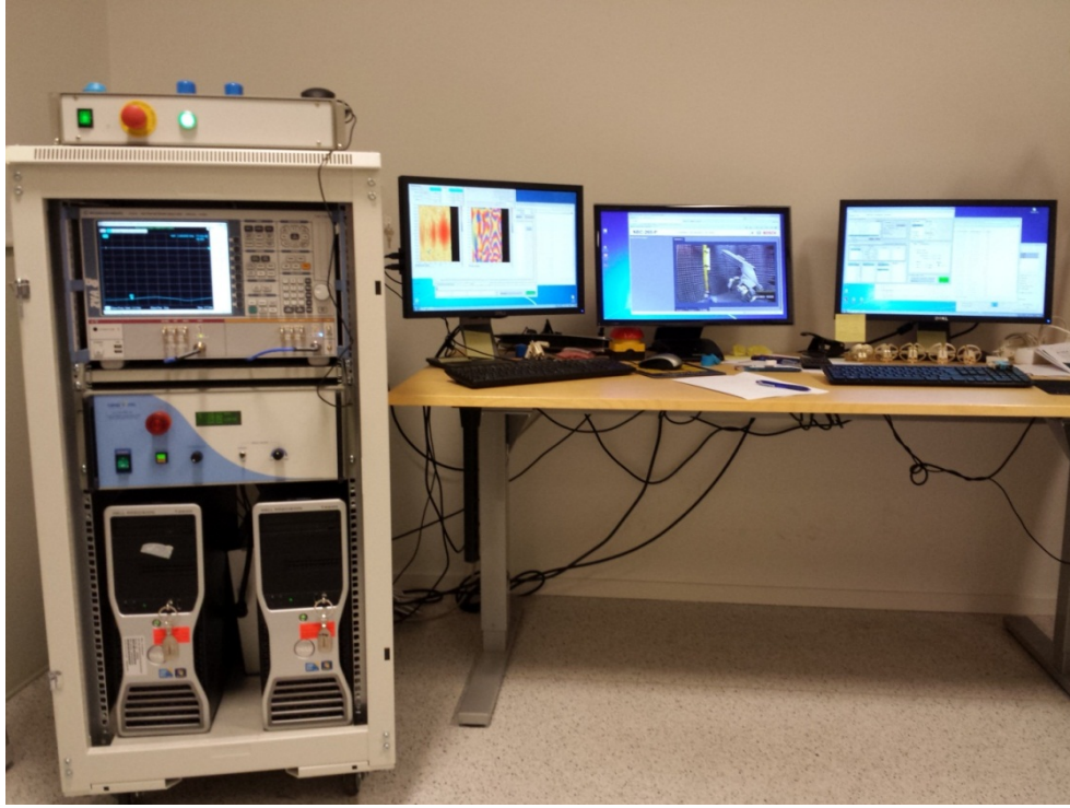
Figure 7. Measurement and analysis equipment for the Orbit/Fr near field system
