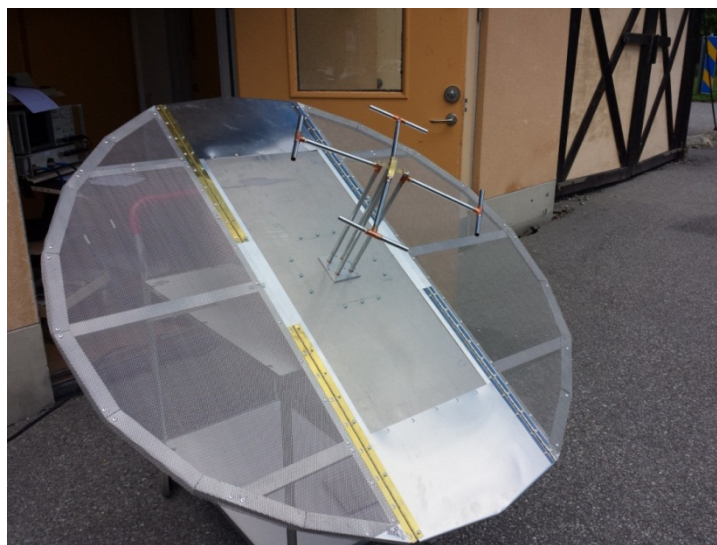
Figure 2. Electrical full-scale model of antenna element no:1 mounted on a ground plane with a diameter of one wavelength ( \lambda ).
